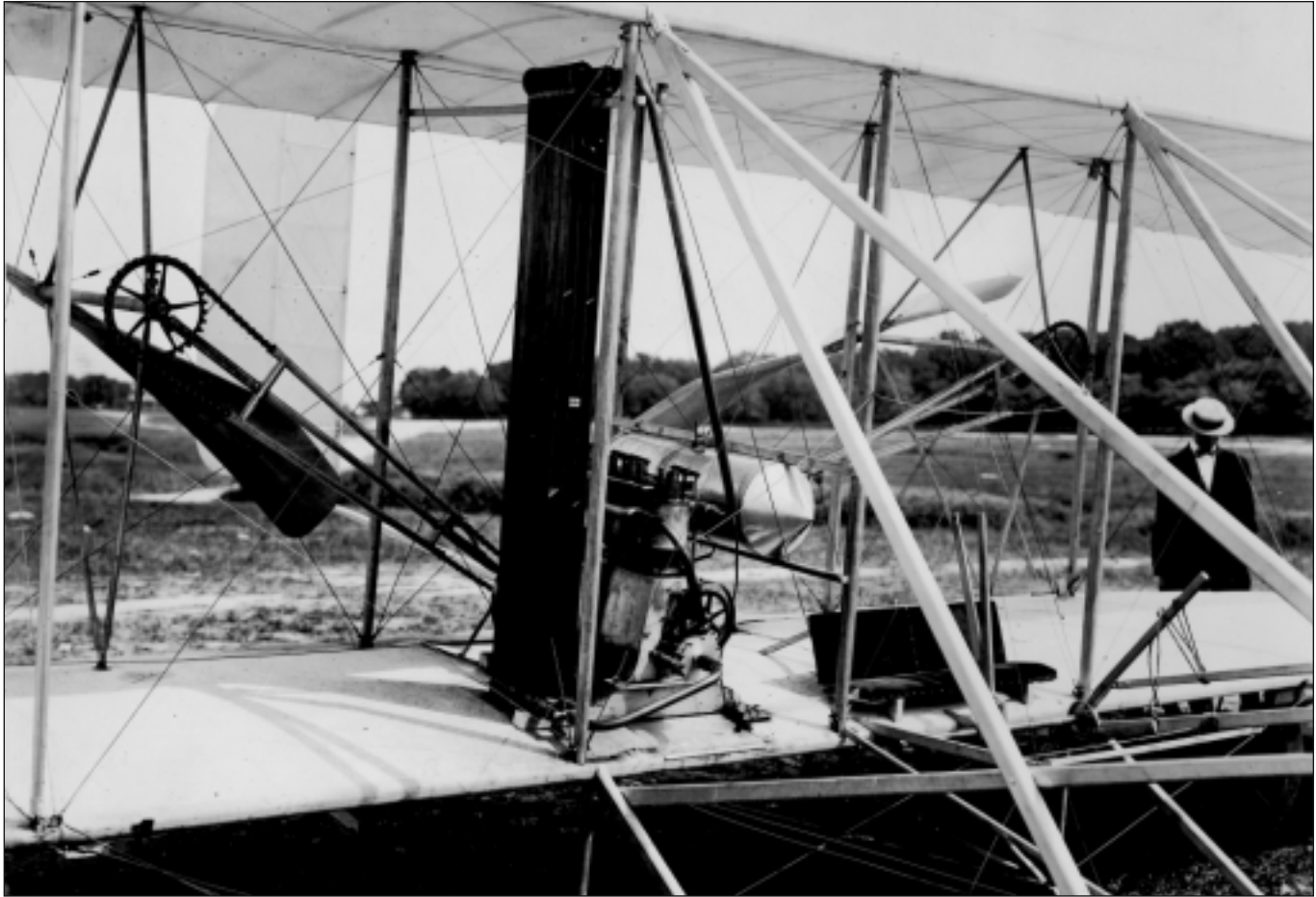
Left-front view of the Wright 1908 Flyer shows the right propeller and chain drive, radiator, engine, fuel tank, seats for the passenger and pilot, and flight-control levers. Orville Wright stands behind the left wing. (Photo: Wright State University)
