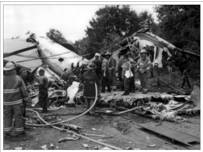
Source: Alan M. Pollack/U.S. National Transportation Safety Board Firefighters examine the tail section of Flight 1016. This section was engulfed by fire.
