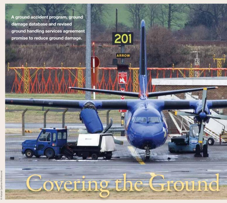
A Fokker F-27-500 engine was damaged in a collision with a towed ground power unit at Edinburgh Airport, Scotland.
