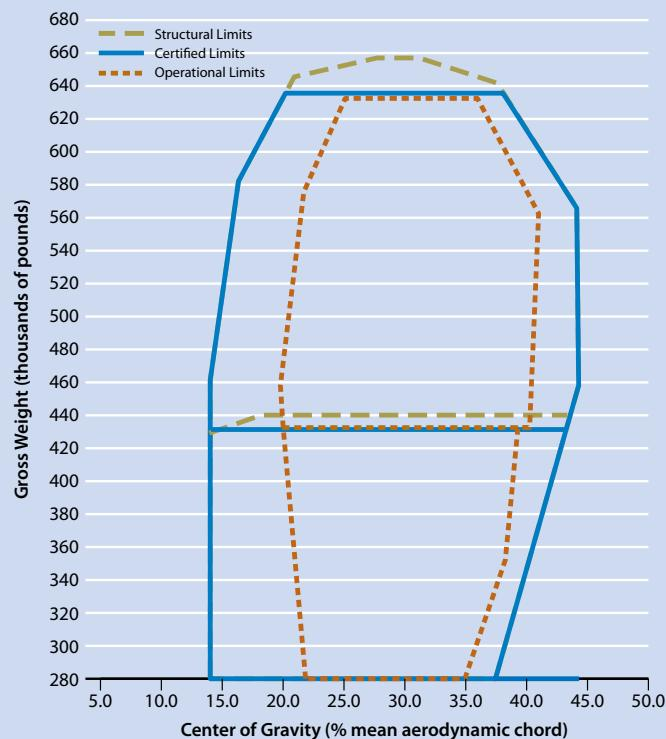
The horizontal lines at 430,000 to 440,000 lb gross weight are the zero fuel weight limits.
