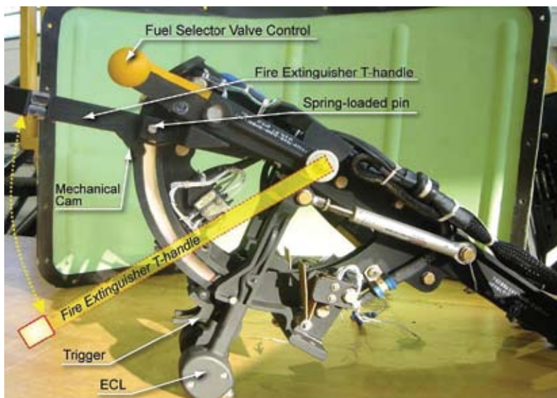
The fire extinguisher T-handle and ECL on an S-76C++
