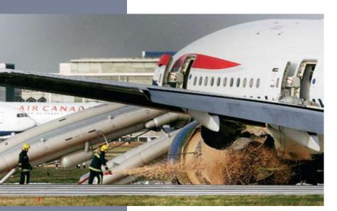
Despite fuel and oxygen leaks, there was no fire. After the brief stabilization, airspeed again began to decrease. As the 777 descended through 200 ft AAL, airspeed was about 108 kt. The stick shaker activated 10 seconds before touchdown, and the copilot pushed his control column forward.
