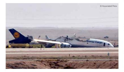
as 3.06 g when the airplane touched down on the nose landing gear following the last bounce."
