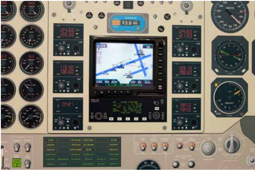
The FAA demonstrates ADS-B with a Garmin Apollo MX20 multifunction display at its technical center in Atlantic City, New Jersey.
