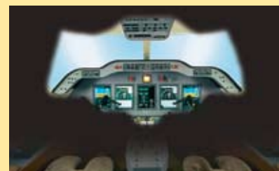
Uncontrolled smoke in the cockpit -Visibility with EVAS
