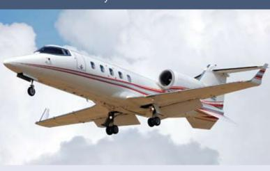
eliveries of the Learjet 60 midsize business jet began in 1993. Compared with its predecessor, the 55C, the 60 has more powerful engines, wing modifications to improve aerodynamic performance, upgraded avionics equipment, a longer fuselage and a larger baggage compartment.
