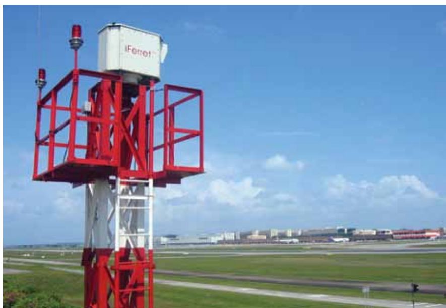
Strattech Systems' iFerret is an electro-optical system that can be used to monitor taxiways and aprons, as well as runways, for FOD.
