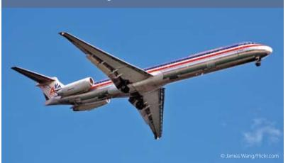
he MD-82 is one of a series of jet transports that are derivatives of the Douglas DC-9, which first flew in 1965. The MD-80 has longer wings, a longer fuselage and more fuel capacity than the DC-9 and an integrated digital flight control system.
