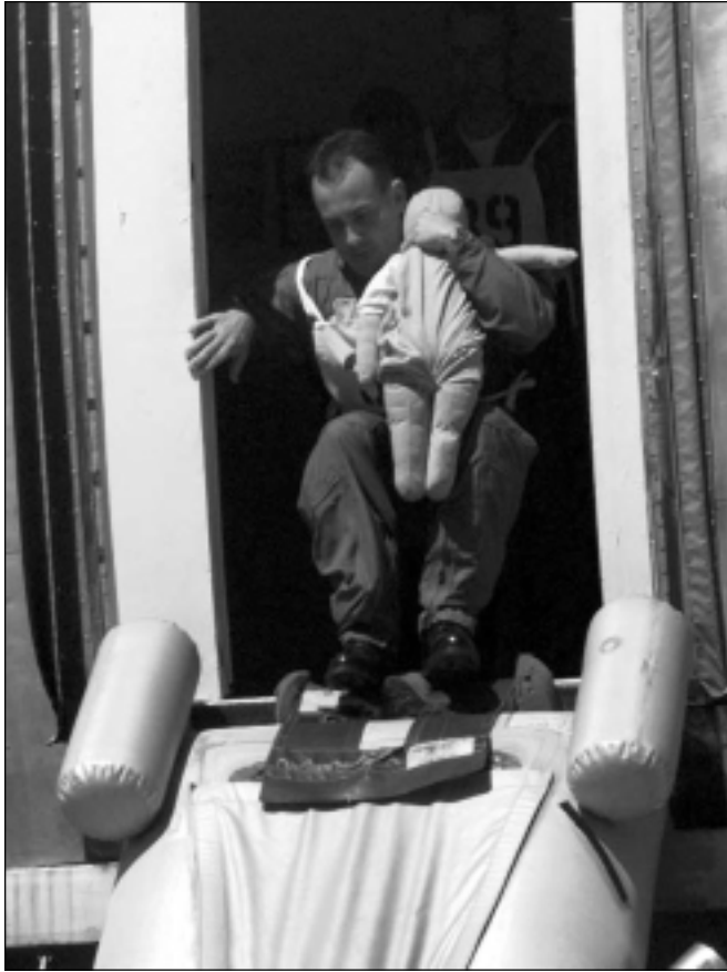
An infant-carrier uses one hand to steady himself as he prepares to sit on an evacuation slide. The infant-dummy is held vertically, and its back is unsupported. (Source: U.S. Federal Aviation Administration Civil Aerospace Medical Institute)
