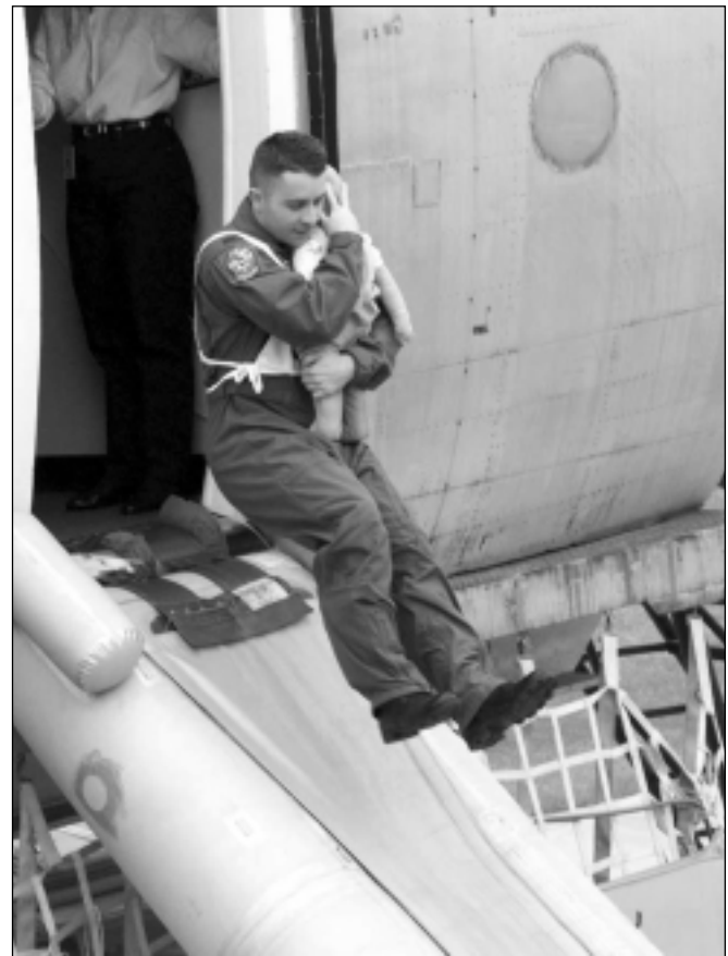
An infant-carrier jumps onto an evacuation slide while holding a dummy representing a six-month old child. The infant-dummy is held vertically, and its head, neck and back are supported. (Source: U.S. Federal Aviation Administration Civil Aerospace Medical Institute)
