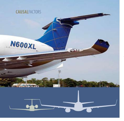
The Legacy pilots experienced control difficulties after the collision but were able to land the airplane. The 737 descended out of control after losing the outer portion of its left wing.
