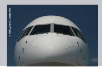
The AD, which affects 1,212 U.S.-registered airplanes, is intended to prevent "smoke, fire or cracking of the inner layer of the forward viewing window," the FAA said, noting that the problem is caused by loose electrical connections designed to heat the windows and prevent icing.
