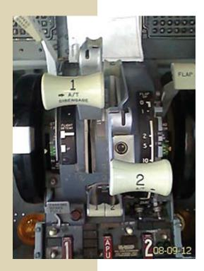
Photo taken on a previous flight shows throttle stagger required to maintain 83 percent fan speed on both engines. hours when the airline began flying it about four months before the accident.
