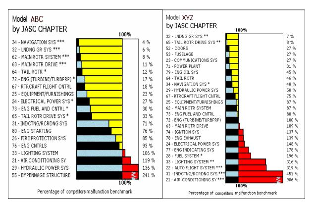
Figure 4 Two Different Models Showing Malfunction Ratios by Mechanical System
