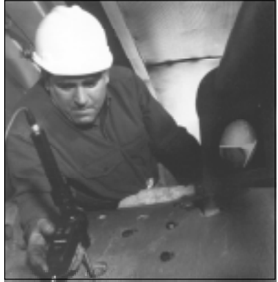
Olympus digital measuring borescope inserted in a gas-turbine access port
