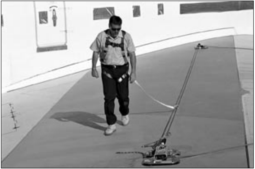
A horizontal lifeline secured to two anchorage connectors helps protect against a fall from an airplane's wing. (Photo: DBI/SALA)
