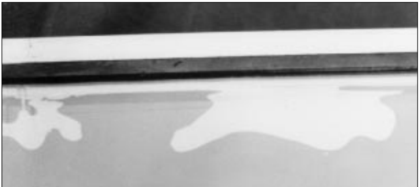
Delamination is a common but repairable type of damage.
