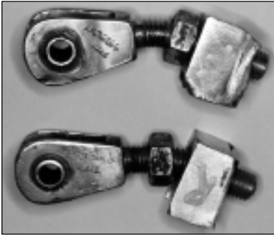
Clevis fittings and mounting blocks were torn from the fairing-panel structure and show the degree of bending overload on the clevis shafts.
