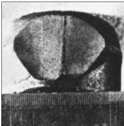
Figure 1. The fracture of the steering drop arm of a motorcar. The width of the arm is approximately one inch.
