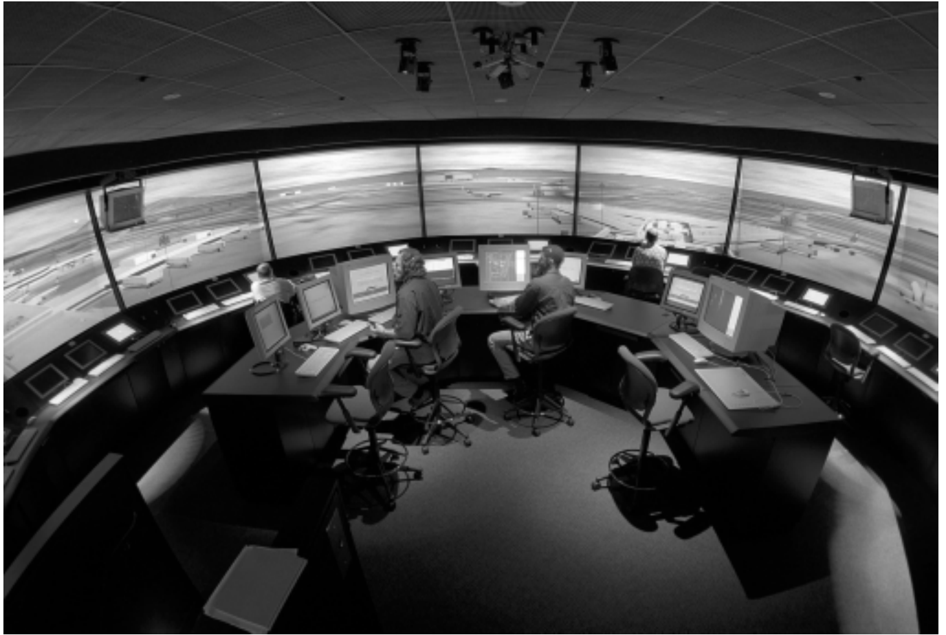
The U.S. National Aeronautics and Space Administration (NASA) FutureFlight Central airport-operations simulator has 12 controller workstations and a 360-degree display of the airport environment. (NASA photo)
