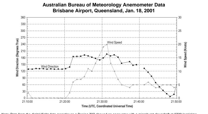
Note: Data from the digital flight data recorder on a Boeing 737 showed an encounter with a microburst downdraft at 0729 local time (21:29 coordinated universal time) and correlated with anemometer data recorded at Brisbane Airport, Queensland, Australia, by the Australian Bureau of Meteorology. High-resolution data from other anemometers at the airport supported air traffic control operations but were not recorded.
