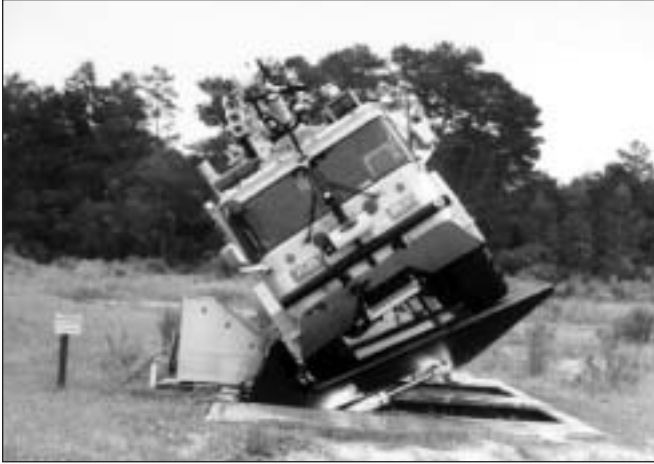
Tilt-table tests alone proved inadequate to evaluate aircraft rescue and fire fighting vehicle resistance to rollover. (U.S. Federal Aviation Administration photo)
