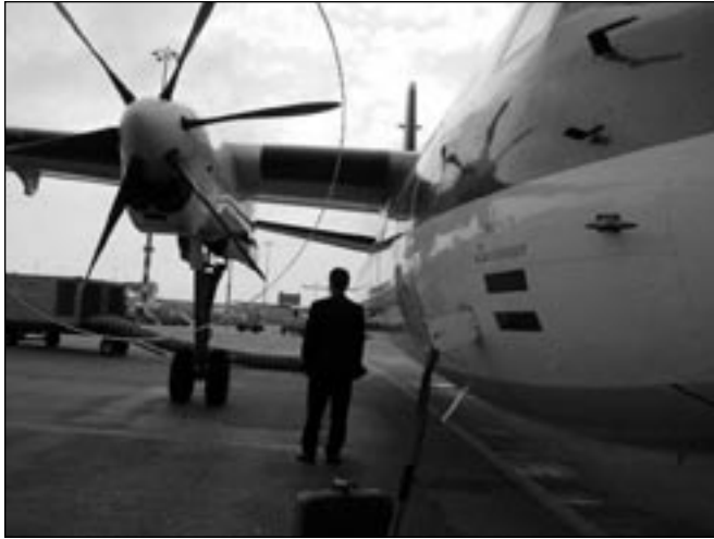
A superimposed arc shows the edge of rotating propeller blades on the Fokker 50. (Source: Dutch Transport Safety Board)
