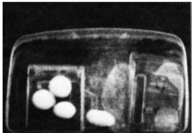
The suitcase on the left contains four balls of C4 plastic explosive. A normal X-ray inspection image of the suitcase barely reveals the shape of only one piece of the explosive; the other three are shielded inside the case of a radio and are not visible. The backscatter X-ray image at the right clearly reveals the four balls of explosive.
