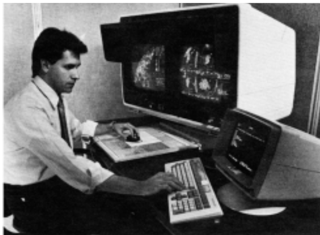
The Principal User Processor (or PUP) for NEXRAD is composed of three main subsystems: the twin color CRT displays; a graphic tablet and "mouse;" and a monochrome terminal and keyboard. Information can be displayed on the color screens using the graphic tablet and buttons on the "mouse." Text on the storm formations are displayed to the right of each display. (Unisys photo)
