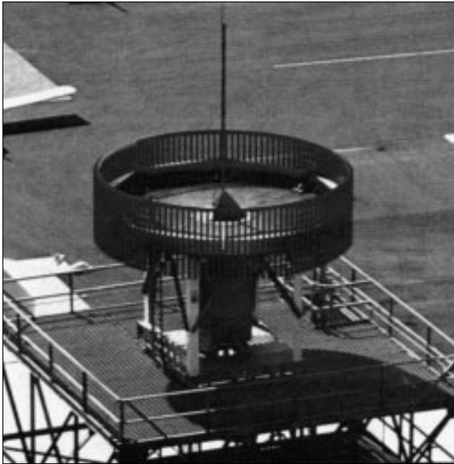
Figure 2. A non-rotating, electronically scanned Parallel/Converging Runway Monitor (PCRM) antenna is computer controlled to provide updates as fast as twice per second in a selected area of interest, such as dual approach courses.
