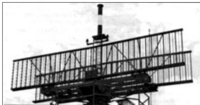
Figure 1. One type of Parallel/Converging Runway Monitor (PCRM) antenna is composed of two rotating open-arrays mounted back-to-back. This doubles the effective scanning speed and provides fast radar screen updates.
