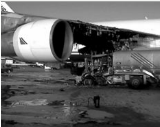
A Boeing 747-259B received substantial fire damage to the right wing during refueling Dec. 1, 1998, at Miami International Airport, Florida, U.S. (Photograph by Timothy Swick)
