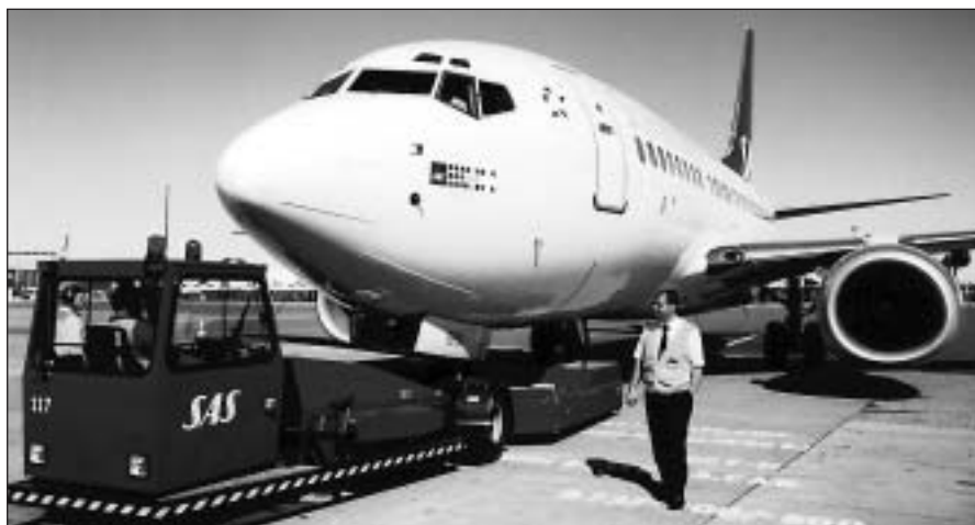
Aircraft pushbacks conducted by one lead agent-driver with a towbarless tractor are among methods preferred by ground-safety specialists.
