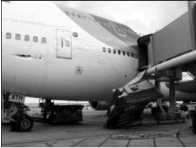
The Boeing 747-300 decelerated in about 12 meters (39 feet) after striking the T1 airbridge at Madrid-Barajas (Spain) Airport, and the rotating roof of the airbridge was embedded in the fuselage. (Spanish Air Accidents and Incidents Investigation Commission photo)
