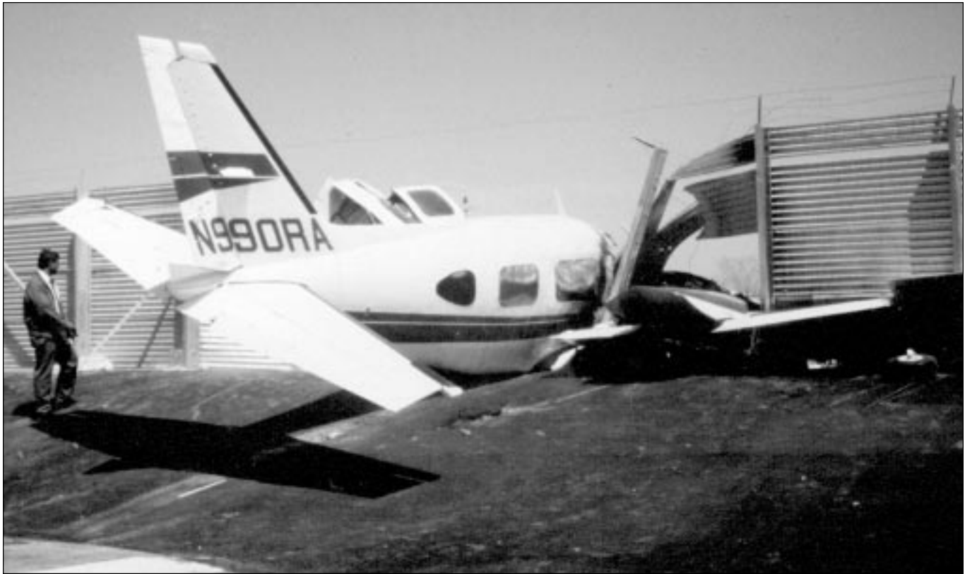
The accident aircraft, a Piper PA-31, impacted a jet-blast fence after landing long. The pilot had elected to make a visual approach despite reduced visibility. The end of the runway is visible in the lower-left corner. (Source: Robert Benzon, U.S. National Transportation Safety Board.)
