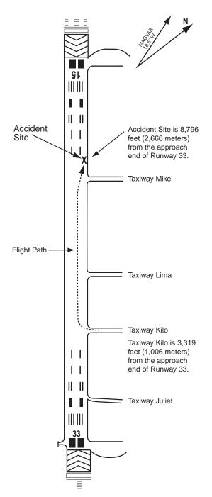
Note: Diagram is not to scale. Runway 33 was 11,439 feet (3,466 meters) long and 300 feet (91 meters) wide. The runway was cleared of snow for its full length; snow had been cleared 150 feet (46 meters) east of the centerline and 75 feet (23 meters) west of the centerline, for a total cleared width of 225 feet (68 meters).
