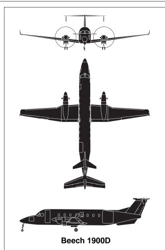
The Beech 1900D is a twin-turboprop regional transport that entered service in 1991 and currently is manufactured by Raytheon Aircraft Co. The airplane is a derivative of the Beech 1900, which first flew in 1982. The 1900D has a flat floor, a maximum cabin height of 5.9 feet (1.8 meters) and 28.5 percent more cabin volume than its predecessor, the Beech 1900C. Standard accommodation is for two flight crew members and 19 passengers.
