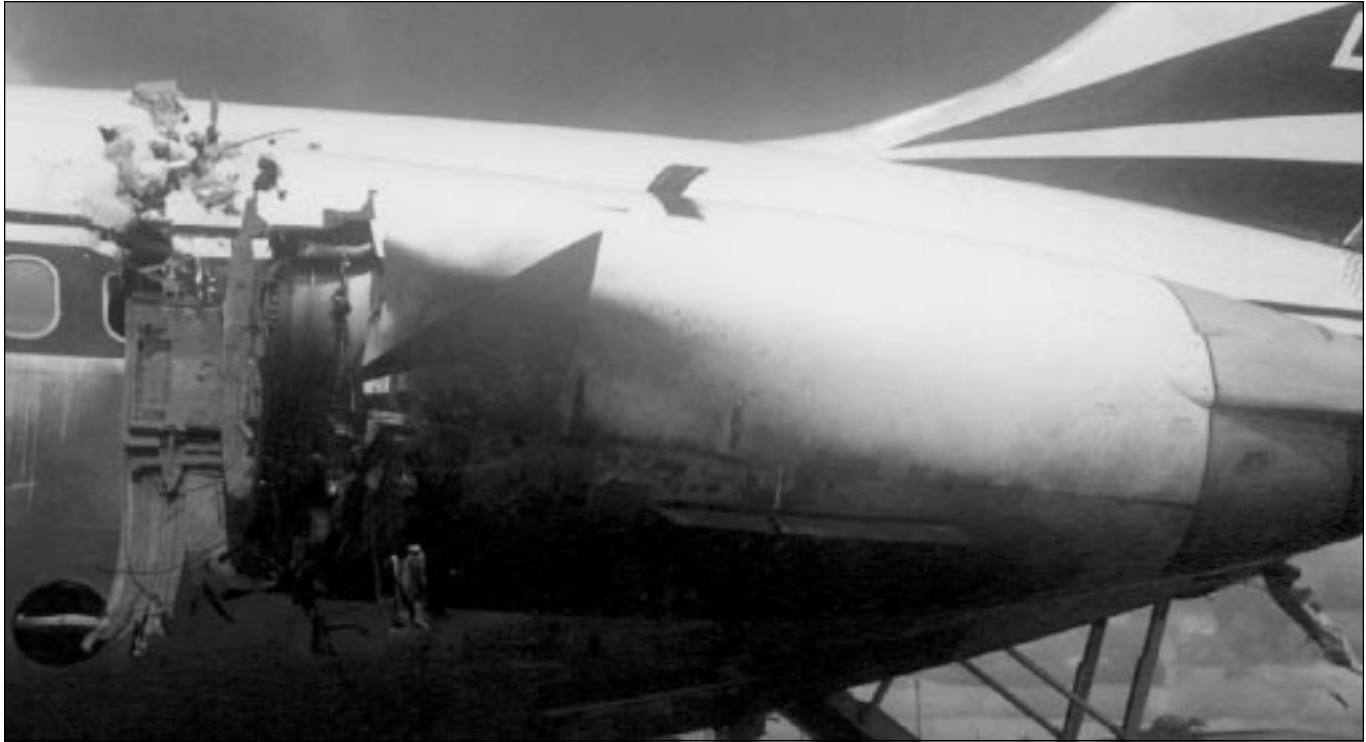
The fan hub and blade assembly of no. 1 engine were separated from the engine in the accident. Debris from the engine penetrated the cabin, killing two passengers and seriously injuring another in the row adjacent to the failed engine. (Photo: U.S. National Transportation Safety Board)
