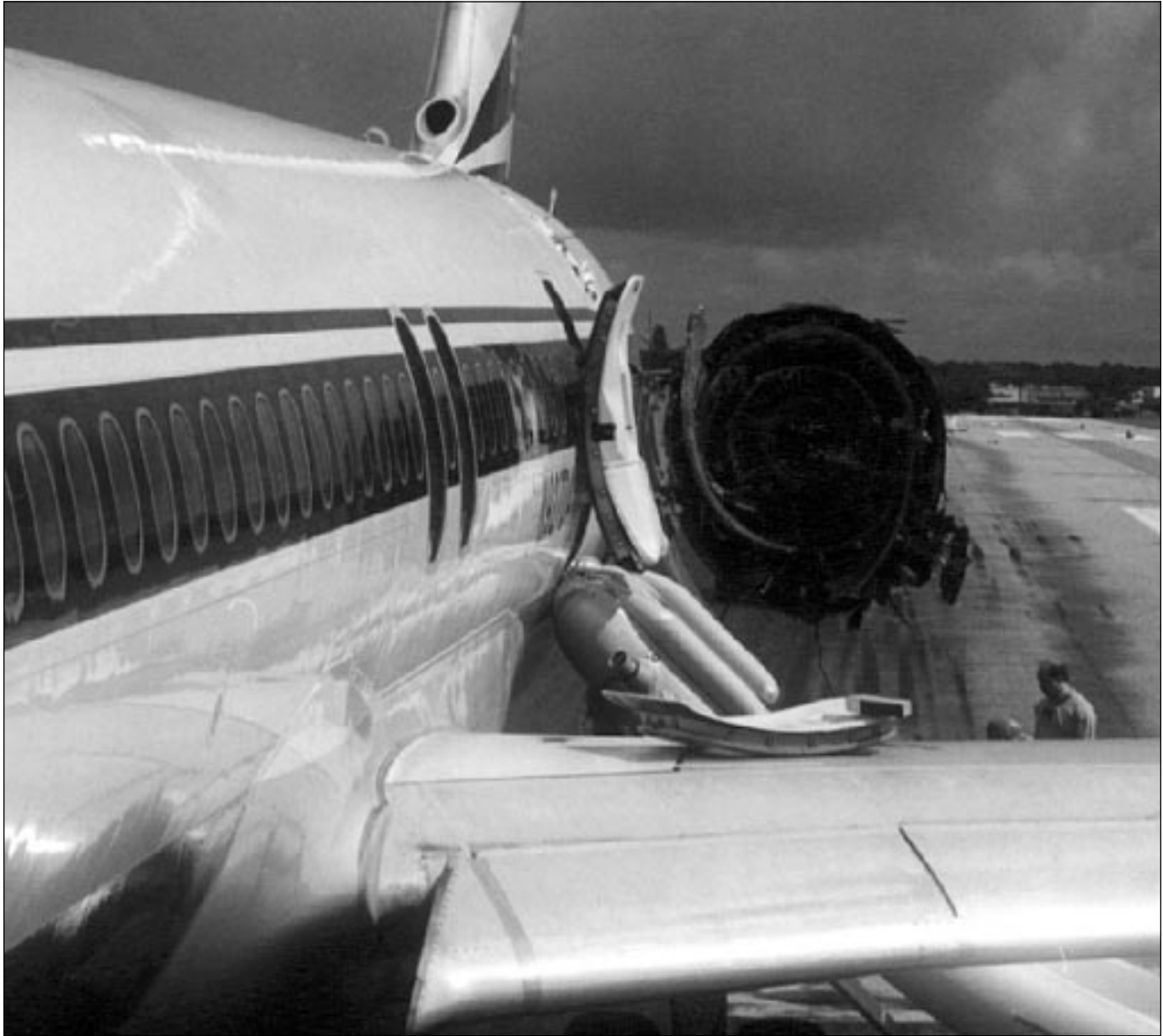
A flight attendant inflated the evacuation slide at the L-2 position, but saw fire on the no. 1 engine's forward cowling and immediately blocked the exit. Evacuating passengers were then directed forward. (Photo: U.S. National Transportation Safety Board)
