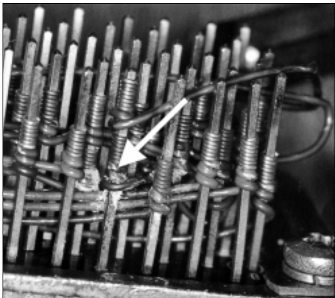
Contamination and corrosion deposits on yaw-damper coupler disrupted electronic signals sent to yaw-damper actuator. (Photo: U.K. Air Accidents Investigation Branch)
