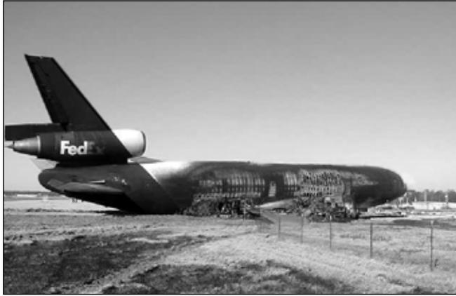
*The left side of the fuselage and the left wing received minimal damage by the impact and fire.* (Photo: U.S. National Transportation Safety Board)
