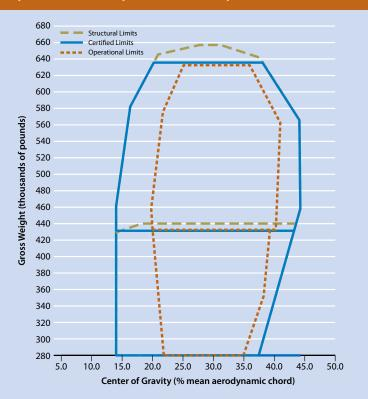
The horizontal lines at 430,000 to 440,000 lb gross weight are the zero fuel weight limits. Source: Patrick Chiles
