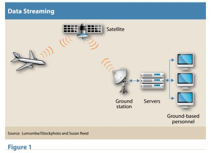
post-flight analysis in cases where the FDR [flight data recorder] cannot be recovered."
