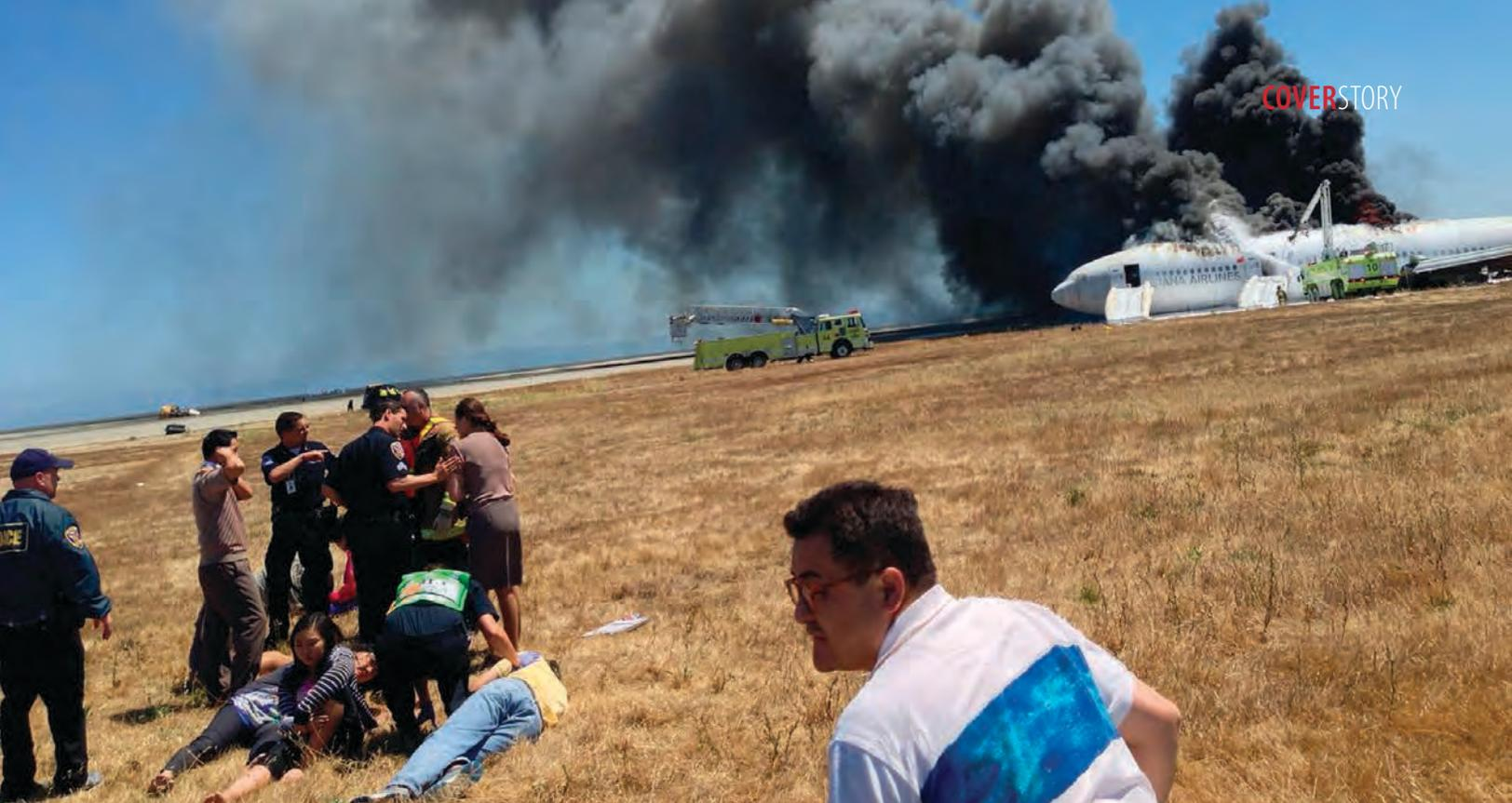
slid along the runway, lifted partially into the air [tilting the airplane into about a 30-degree nose-down angle], spun about 330 degrees, and impacted the ground a final time [coming to rest off the left side of the runway, about 2,400 ft (732 m) from the initial seawall impact point ... about 1128:06.26 local time].
