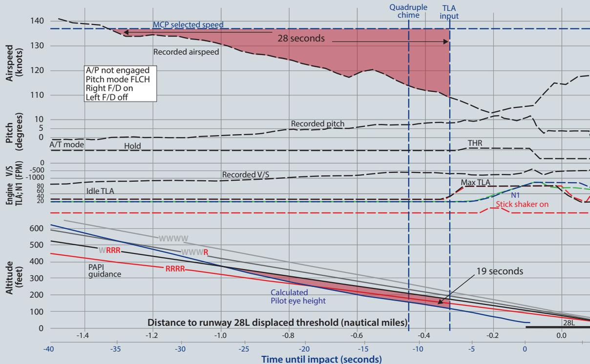
A/P = autopilot; A/T = autothrottle; F/D = flight director; FLCH = flight level change; FPM = feet per minute; MCP = mode control panel; N1 = engine low pressure spool speed; PAPI = precision approach path indicator; THR = thrust; TLA = throttle lever angle; V/S = vertical speed
