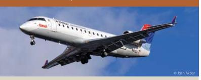
he Canadair Group of Bombardier in 1987 began design studies based on the Challenger business jet for the Canadair Regional Jet (CRJ). The first model, the CRJ100, entered service in 1992. The 50-passenger airplane is powered by General Electric CF34-3A1 engines flat-rated at 9,200 lb (41 kilonewtons).
