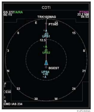
The cockpit display of traffic information shows the own ship as a blue triangle merged behind the UPS2 airplane and actively controlling its speed to maintain proper in-trail spacing.
