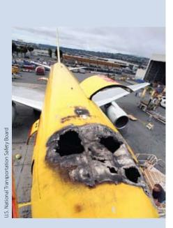
The NTSB also recommended that ABX Air "modify [its] continuing analysis and surveillance program so that all identified chronic discrepancies, such as those affecting the oxygen system on the accident airplane, are effectively resolved."
