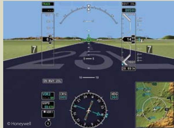
This integrated primary flight display gives pilots situational awareness of the flight path, terrain and navigational environment.
