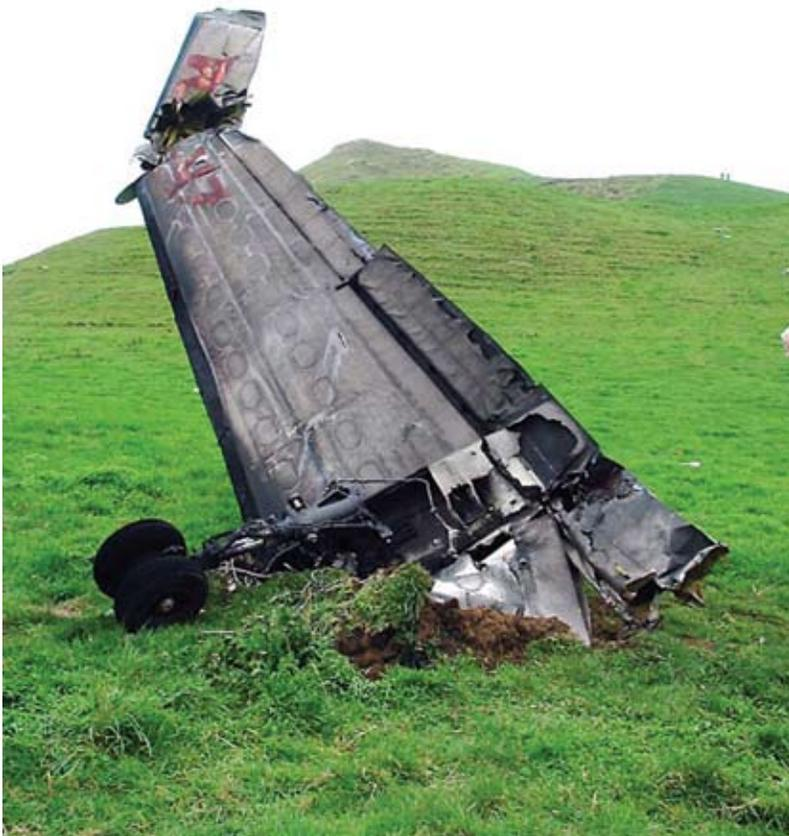
The CVR recorded the sounds of power reduction about seven seconds before the recording ceased. “This was late in the development of the spiral dive, and the delay would have exacerbated the situation,” the report said.
