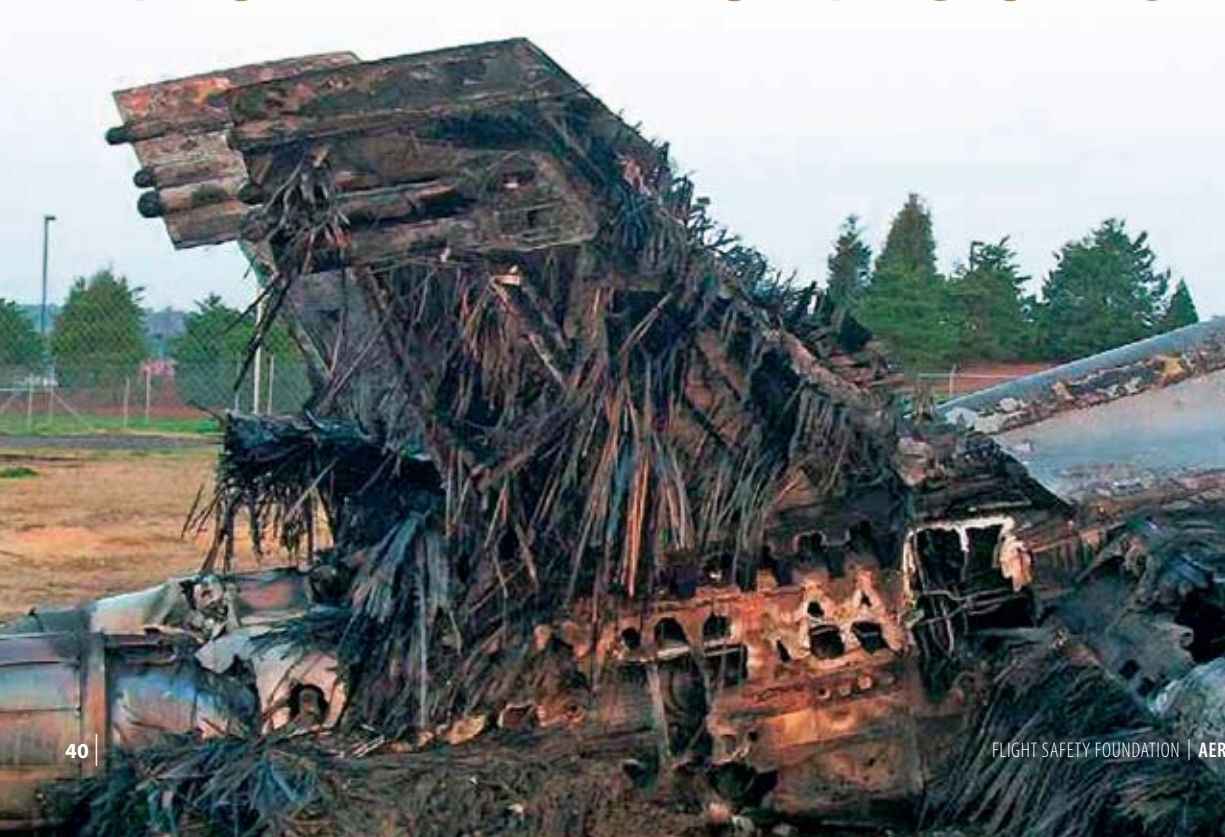
Fire damage to an F/A-18 Hornet fighter illustrates fiber composite debris.
