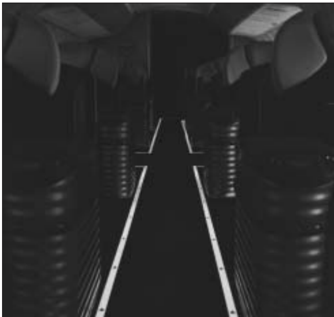
The green glow of photoluminescent strips or tracks along both sides of aisles becomes readily visible in darkness. (Lufthansa Technik photos)
