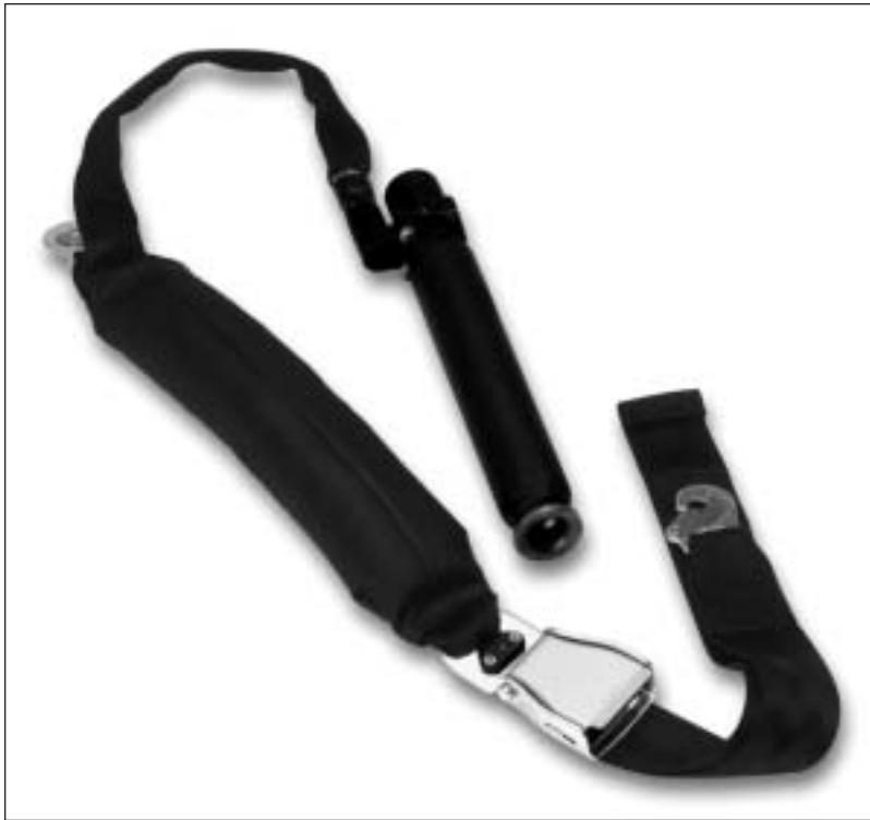
The sheath attached to one end of the seat belt contains an inflatable nylon bag, connected to the inflator (the cylindrical object in the center). When installed, the inflator is out of view under the passenger seat. (Amsafe Aviation photo)
