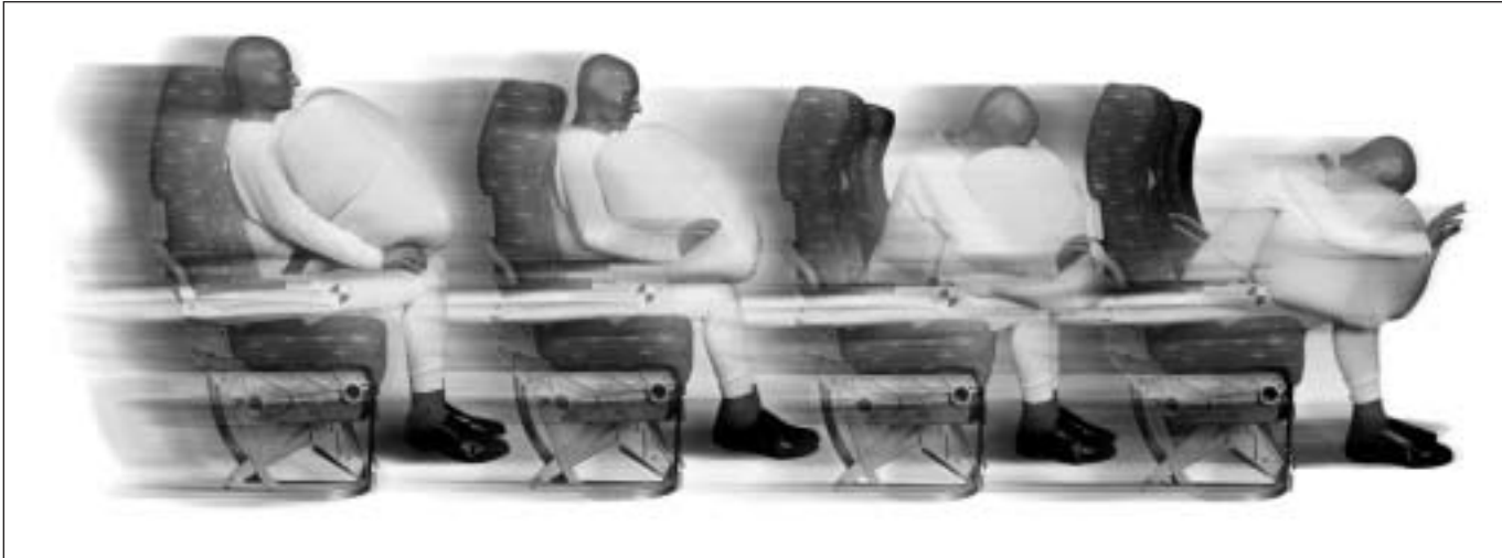
In this sequential view, the inflated bag absorbs the energy of the anthropomorphic test dummy articulating forward in a simulated accident scenario. (Amsafe Aviation photo)
