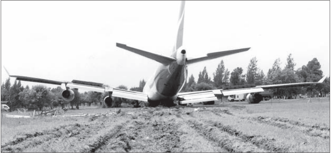
Substantial damage to the Boeing 747-400 during the runway overrun included collapse of the nose gear and the right-wing landing gear. The aircraft was in a nose-low position and a slightly right-wing-low position during the precautionary disembarkation. (Australian Transport Safety Bureau Photo)
