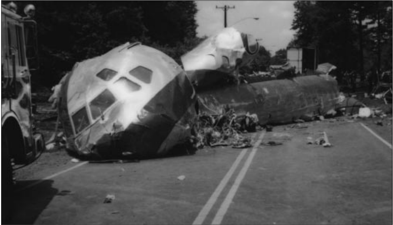
The nose of Flight 1016 sheared off on impact with trees and skidded down a residential street. Another section of the fuselage is behind the nose section. (Source: Allan M. Pollock/U.S. National Transportation Safety Board.)
