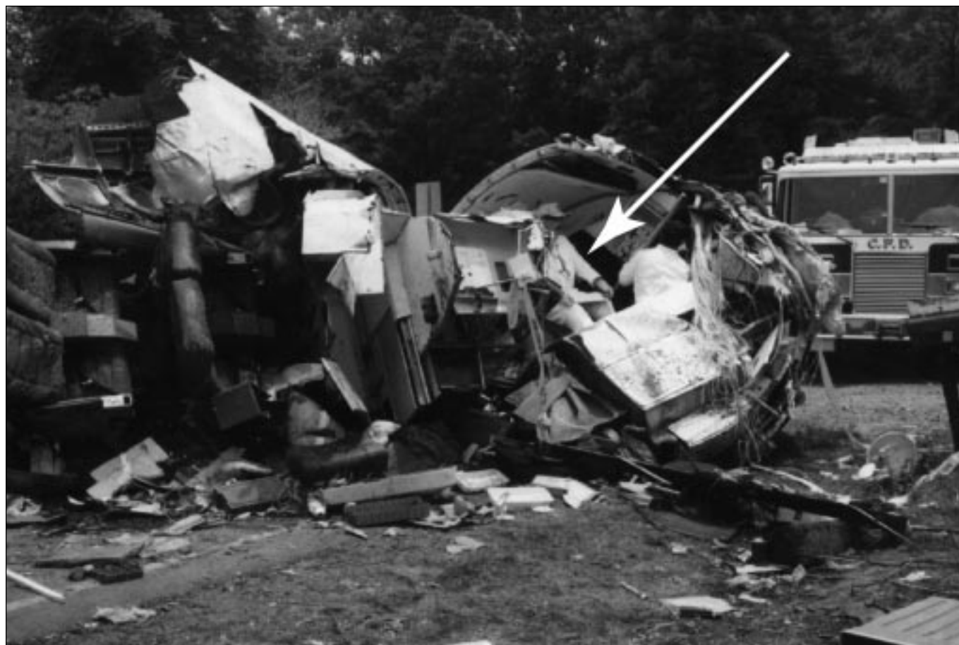
A view from the rear of the destroyed nose section and of the area where flight attendants DeMary and Markwith were seated (marked by the arrow) at the time of the crash. (Source: Alan M. Pollack/U.S. National Transportation Safety Board.)
