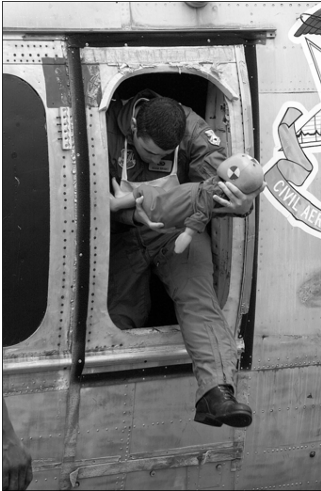
An infant-carrier holds a dummy of an 18-month-old child in a horizontal position, using both hands to support its head and body, while evacuating the airplane. (Photo: U.S. Federal Aviation Administration Civil Aerospace Medical Institute)
