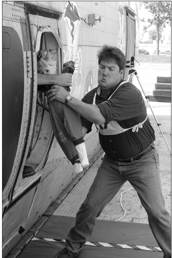
A dummy of a 24-month-old child is passed through the exit to a study participant. (Photo: U.S. Federal Aviation Administration Civil Aerospace Medical Institute)
